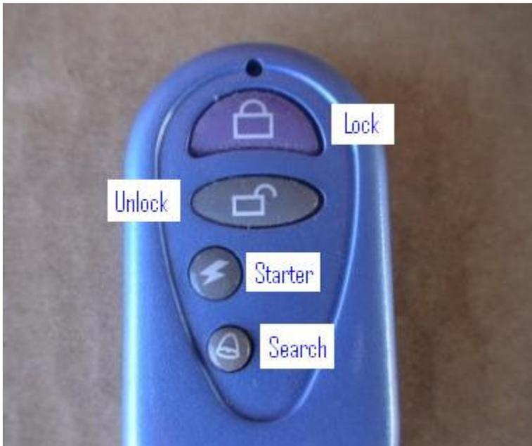
There are 4 press buttons in each remote, as shown in the picture 11 above. These 4 press buttons are referred to LOCK, UNLOCK, STARTER, and SEARCH buttons for description of operation followed.
